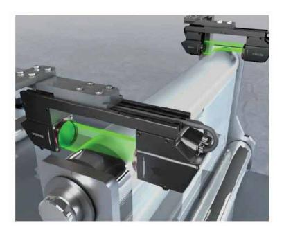
Online Thickness Measurement System for Looper
